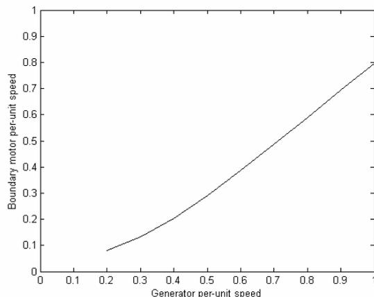
Fig. 5. Relationship between the generator per-unit speed and the boundary value of the motor speed.
