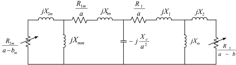
Fig. 2. Equivalent circuit of SEIG / IM system
